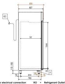
ED Remote electrical connection RO ΕI Electrical inlet (power) Refrigerant Inlet
